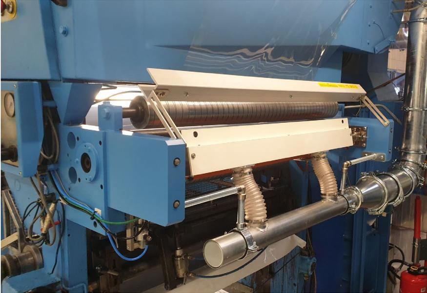
**Xstream high velocity non-contact surface cleaning system with AUTO DC Technology® ionising system**
