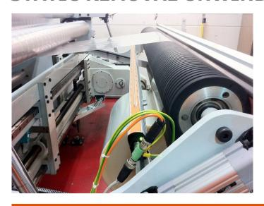
**iON**stream 4.0 network capable AUTO DC Technology® static neutralising system
