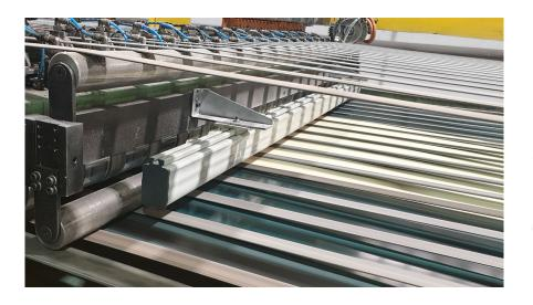
iONstream 4.0 network capable AUTO<sup>DC</sup> Technology<sup>®</sup> static neutralising system
