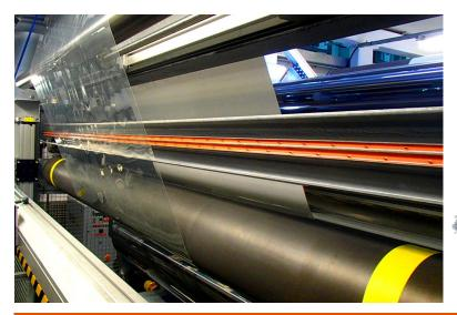
iONstream 4.0 network capable AUTO DC Technology<sup>®</sup> static neutralising system
