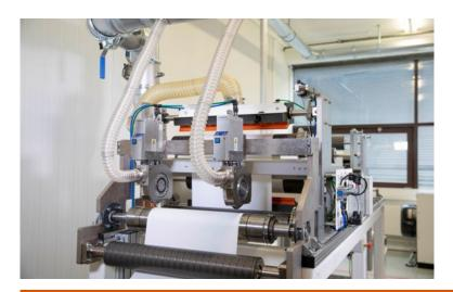
In order to meet the increased demand for demonstrations and customer trials - *extraction of cut-off dust* - the test facility in our customer laboratory was equipped with 2 pneumatic Dienes knife holders and cut-off dust extraction **SLITstream** system from Hildebrand Technology.
