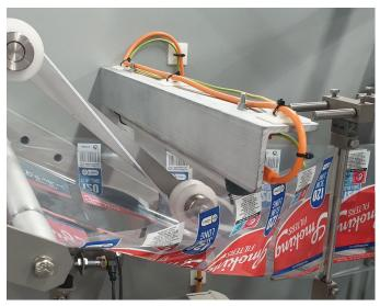
iONstream 4.0 network capable AUTO DC Technology® static neutralising system
