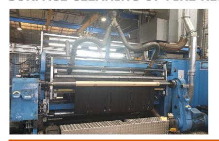
Xstream high velocity non-contact surface cleaning system with AUTO DC Technology® ionizing system
