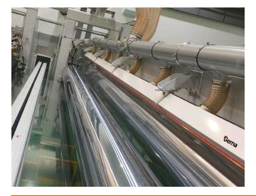
Xstream high velocity non-contact surface cleaning with AUTO DC Technology<sup>®</sup> ionizing system for PP/PE and PTFE film of 2-400µm
