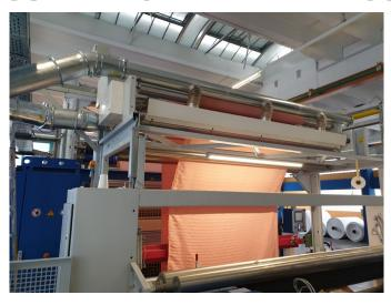
Xstream high velocity non contact surface cleaning technology with AUTO DC Technology® ionisation system
