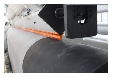
Xstream high velosity non contact surface cleaning technology with AUTO<sup>DC</sup> ionisation system
