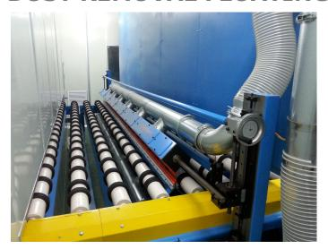
**Xstream** high velosity non contact surface cleaning technology with AUTODC ionisation system
