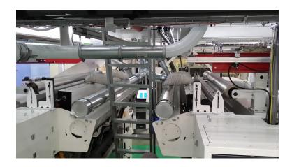
Xstream high velocity non contact surface cleaning technology with AUTO<sup>DC</sup> ionisation system
