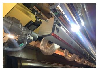
Xstream XL-Modular high speed non contact surface cleaning technology with AUTODC ionisation system
