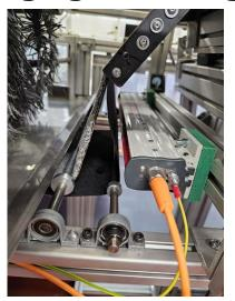
With the 20kV ioncharge 4.0 electrostatic charging system textile and carpet materials can be easily charged for temporary attachment, before fastening.
