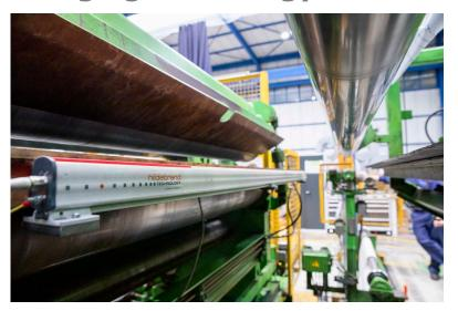
With the 20kV iONcharge 4.0 high voltage generator even paper materials can be easily charged for temporary fixation on metal
