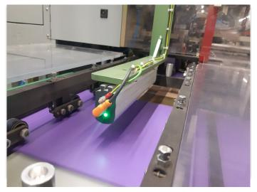
With the 20kV iONcharge 4.0 high voltage generator film and plastic materials can be easily charged for temporary fixation, during lamination.
