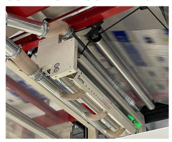
Xstream high velocity non-contact surface cleaning with AUTODC® ionising system
