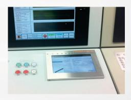
iONstream Fusion can be controlled and monitored by iONpilot Industrial APP, which enables a direct access to the data parameters of the discharging and cleaning process via touch-panel.
