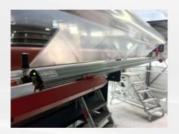
iONstream Fusion is a microcontroller driven static neutralizing system with an integrated onboard high voltage generator. The heart of the neutralizing technology is the patented 'Auto DC' operation mode. The system automatically adapts the correct discharging polarity and neutralizes the charged substrate in a most possible perfect efficient way. When working in potentially
