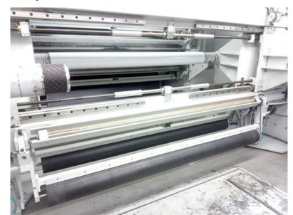
1 x **iONstream 4.0**, 6kV, 2600 mm in (Ex) version 1 x **iONstream 4.0**, 12kV, 2600 mm
