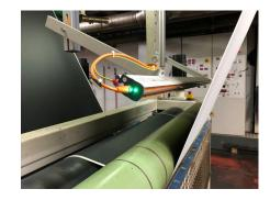
iONcontrol industrial panel connected to several iONstream 4.0 network capable AUTO DC Technology® ionisation bars
