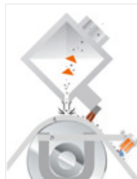
Nozzle principle Xstream
